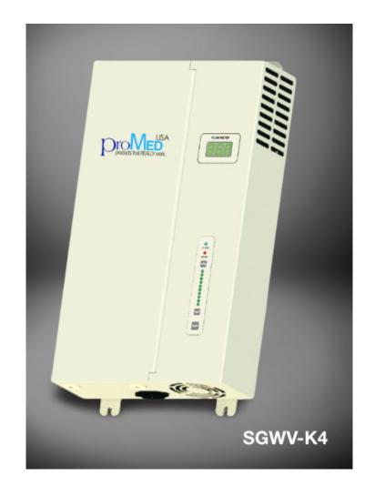
The ProMedUSA Model SGWV-K4 Series Ozone Generator is a small, lightweight wall mounted unit that can produce 4gm/hr of ozone with a dry air feed, and 7gm/hr of ozone with an oxygen feed.
